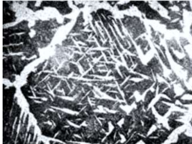
1 – v – fig. Image of St3G sp alloy magnified x2000
