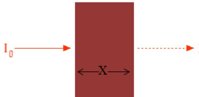
**Figure 1: Attenuation of beam of gamma ray through an absorber of thickness (X) [14]**
