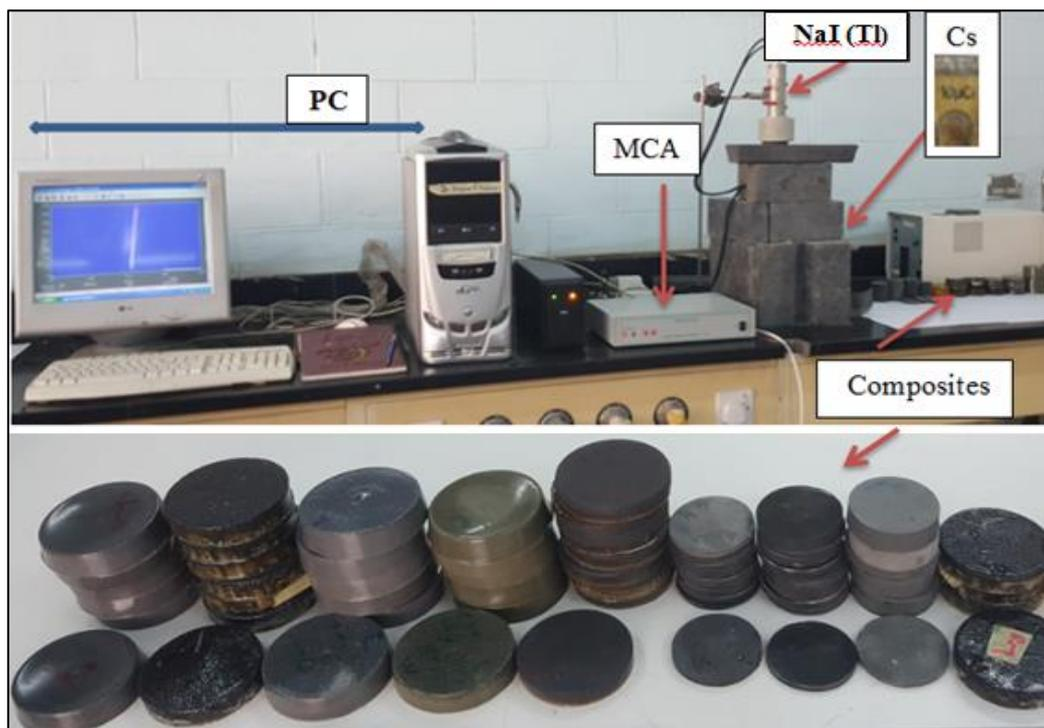
Figure 3: experimental setup arrangement Baghdad University Nuclear Laboratory.
