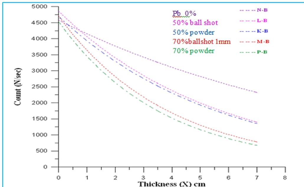
**Figure 4: Relation between count per second as function for thickness**
