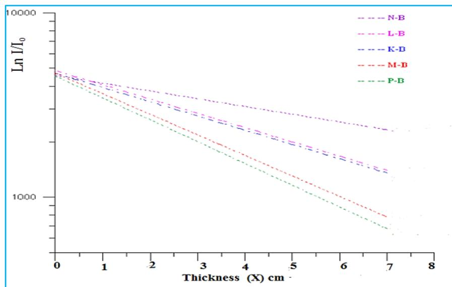
**Figure 5. Shows ( $\ln I/I_0$ ) as a function of thickness of the Composites shields**
