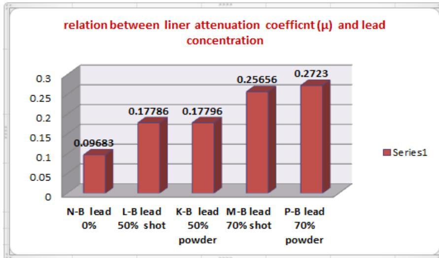
**Fig .6 relation between linear attenuation coefficient ( $\mu$ ) and lead concentration**
