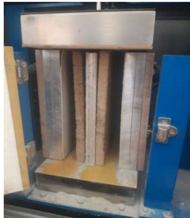
3-picture. Determination of heat transfer coefficient of vermiculite plate obtained on the basis of multiplied vermiculite (on XND-2-3030C machine).
