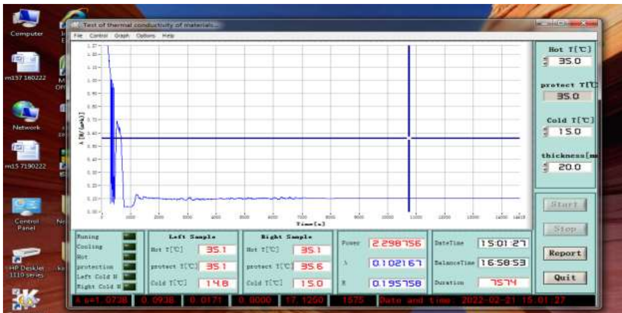
4-picture. Determination of heat transfer coefficient of vermiculite plate obtained on the basis of multiplied vermiculite (on XND-2-3030C machine).
