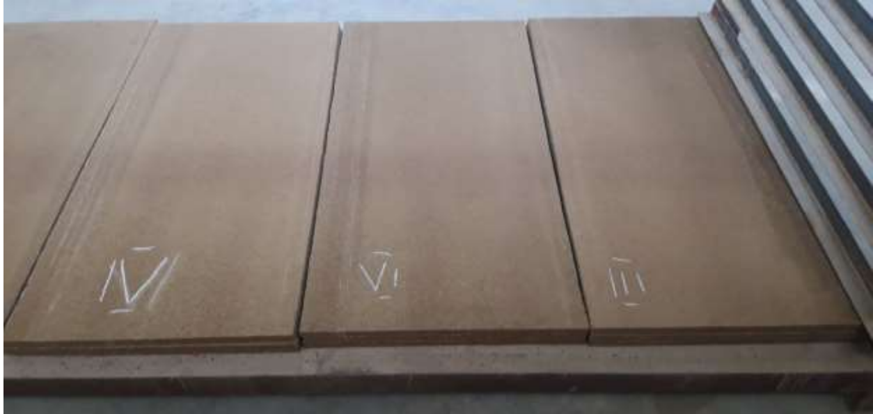
2-picture. Vermiculite plate made on the basis of multiplied vermiculite prepared on the basis of experimental works .
