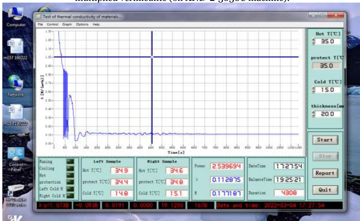
6-picture. Determination of heat transfer coefficient of vermiculite plate obtained on the basis of multiplied vermiculite (on XND-2-3030C machine).
