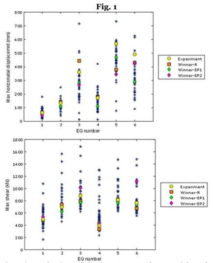
Predictions of maximum horizontal displacements at the top of the column and maximum base shears versus measured values (Terzic et al. <u>2015</u>)
