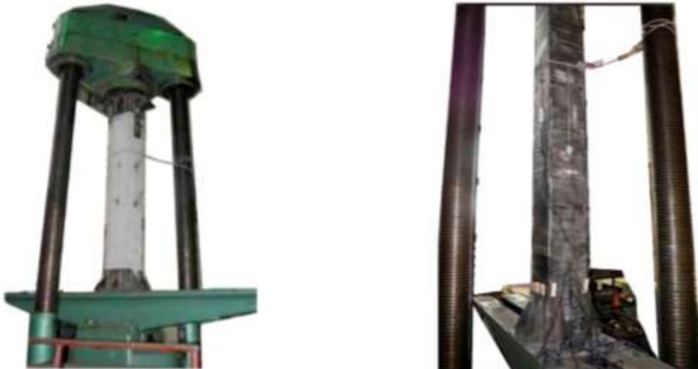
Figure 5. The process of testing an unreinforced (left) and canvas-reinforced (right) reinforced concrete column (source [5])
