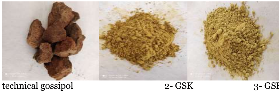
Figure 4. 2-GSK, 3-GSK formed after degreasing technical gossypol crystallization steps The chemical reactions of precipitation of gossypol with acetic acid are shown in Scheme 3.
