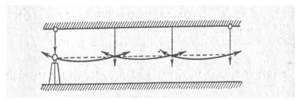
performed in an orderly manner: theodolite is centered, horizontal and vertical angles are measured, the length between the points is measured in the correct and opposite direction, and the lengths from point to right, left, ship, and bottom are measured using ribbons along the theodolite path.
