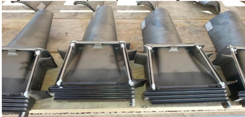
Figure 8 Preparing the blades before installation
