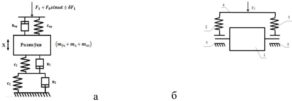
here, 1 – roller, 2,3 – springs, 4 – body plate, 5 – roller supports.
